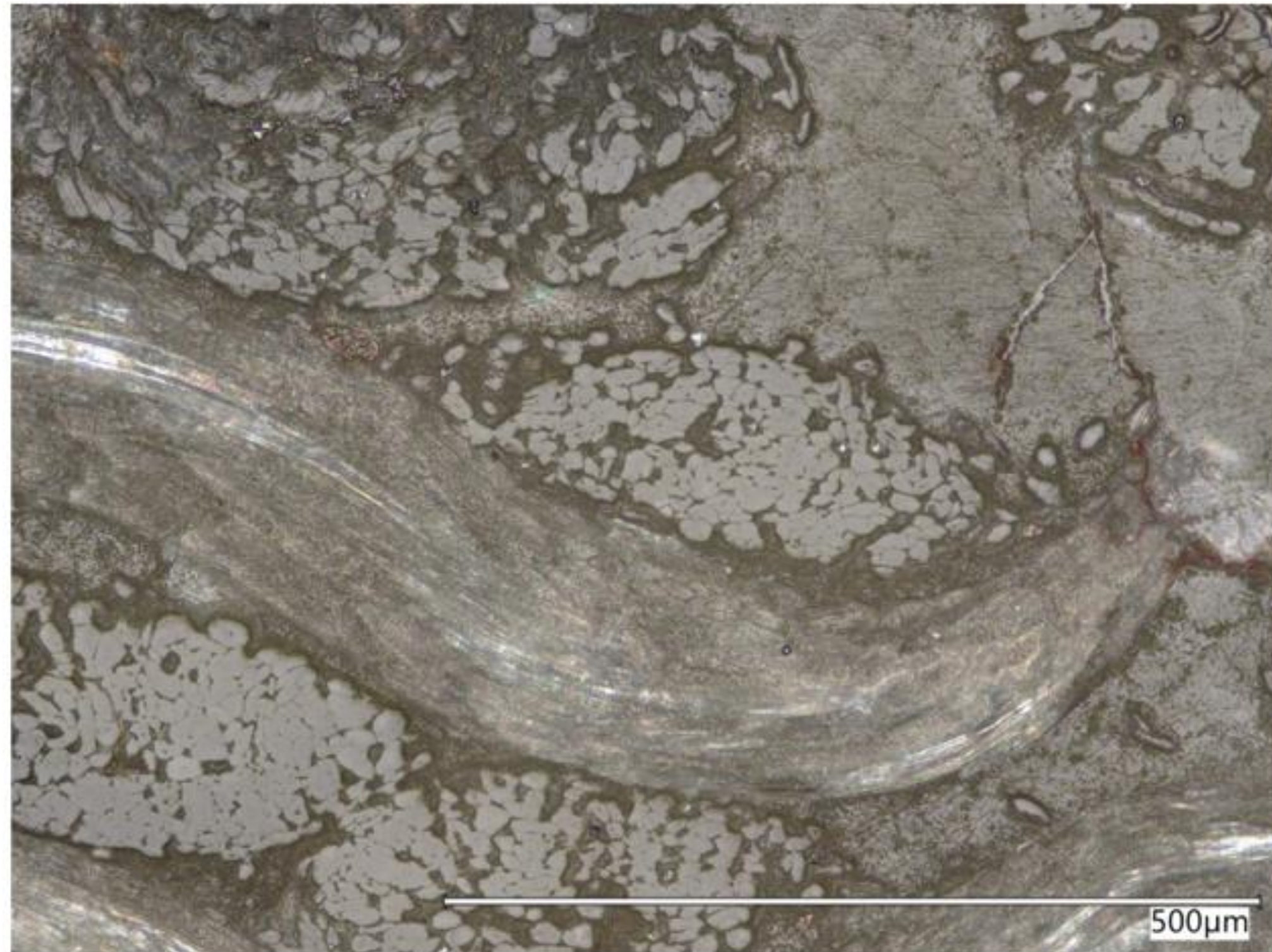
Optical microscopy of Hemp Weave/PLA composite at 400\times magnification (left) and segmented fiber object masks obtained with micro-SAM (right).
