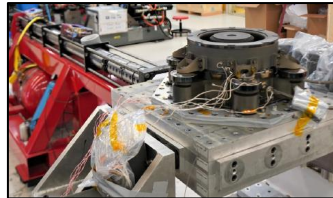
QM-1 Thruster undergoing lateral shock test.
