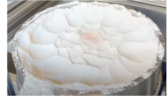
Direct concentrated solar on Greenspar 250 simulant didn't melt, only slightly sintered.
