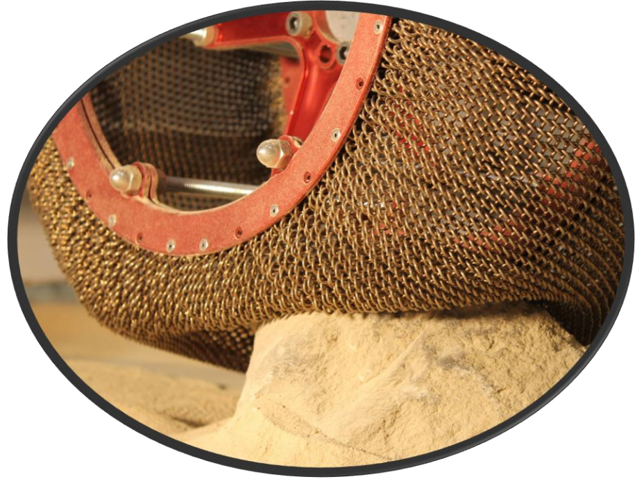
Superelastic components for extreme environments: lunar rover tires, bearings
