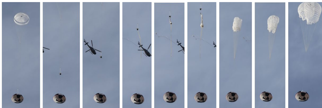
Figure 13 - Developmental Drop Test Main Parachute Deployment Sequence
