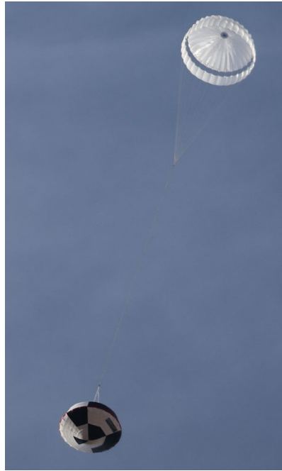
Figure 2 - Dragonfly 8.25m Do Drogue Parachute
