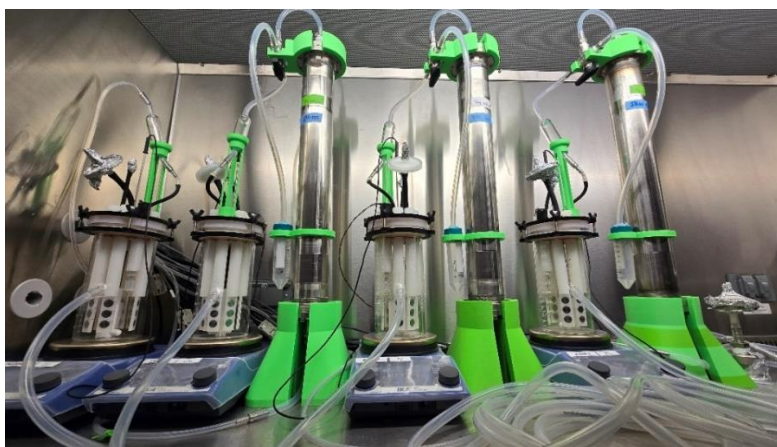
Figure 9. Nutrient canisters integrated into the Biofilm Test Stand. IRC 120 (left), BFR 300 (middle), and IRN 150 (right)
