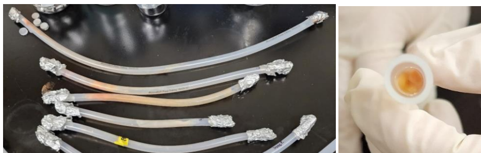
Figure 3. Clogged drain tubing from all bioreactors (left) and a fully occluded drain tube from bioreactor 3 (right).
