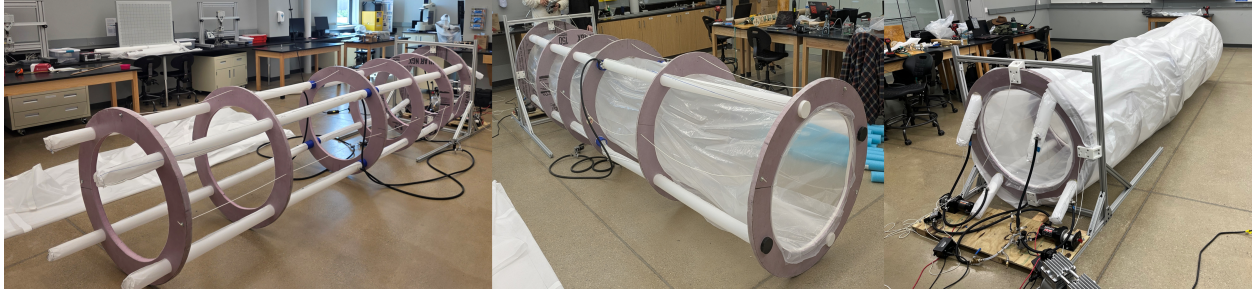
Figure 17: Evolution of the final tunnel prototype. Left: The fiberglass-reinforced foam ribs supported by pressurized bladders. Middle: Plastic sheeting added to the tunnel to serve as internal walls. Right: Final tunnel prototype with nylon outer shell.
