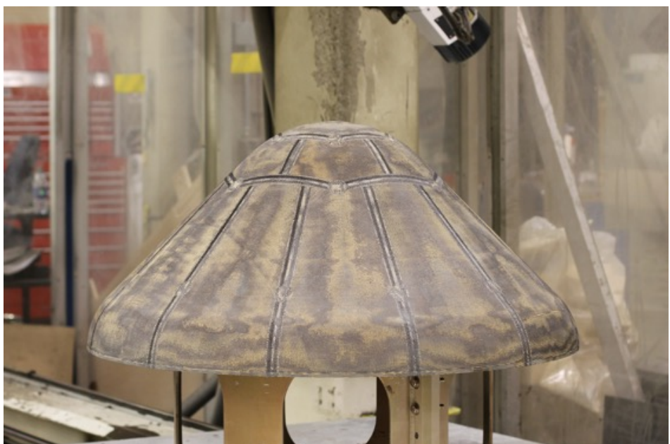
HEEET 1m diameter, 45° sphere cone Engineering Test Unit
