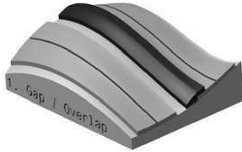
Figure 2.2: 3D graphical representation of a gap/overlap [18].
