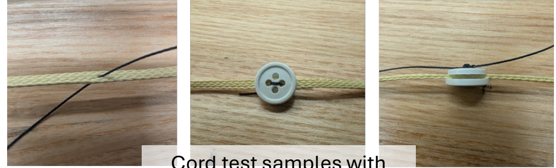
Cord test samples with sewn button targets
