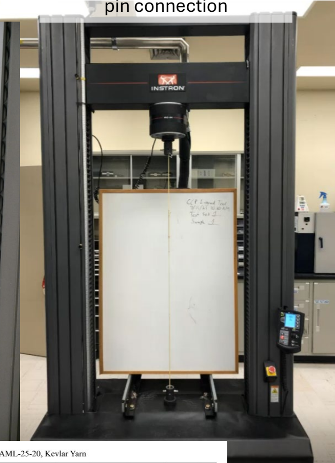
Instron Machine with pin-to-pin connection
