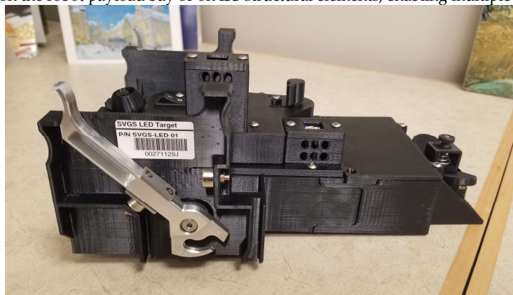
Figure 2. The flight-qualified SVGS tetrahedral beacon (Rev. 8) includes a DC-DC converter, LiPo battery, and overdischarge protection circuitry. A dimmer allows adjusting to different illumination conditions within the ISS environment.
