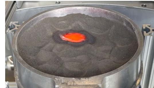
Direct concentrated solar on JSC-1A simulant melted within seconds
