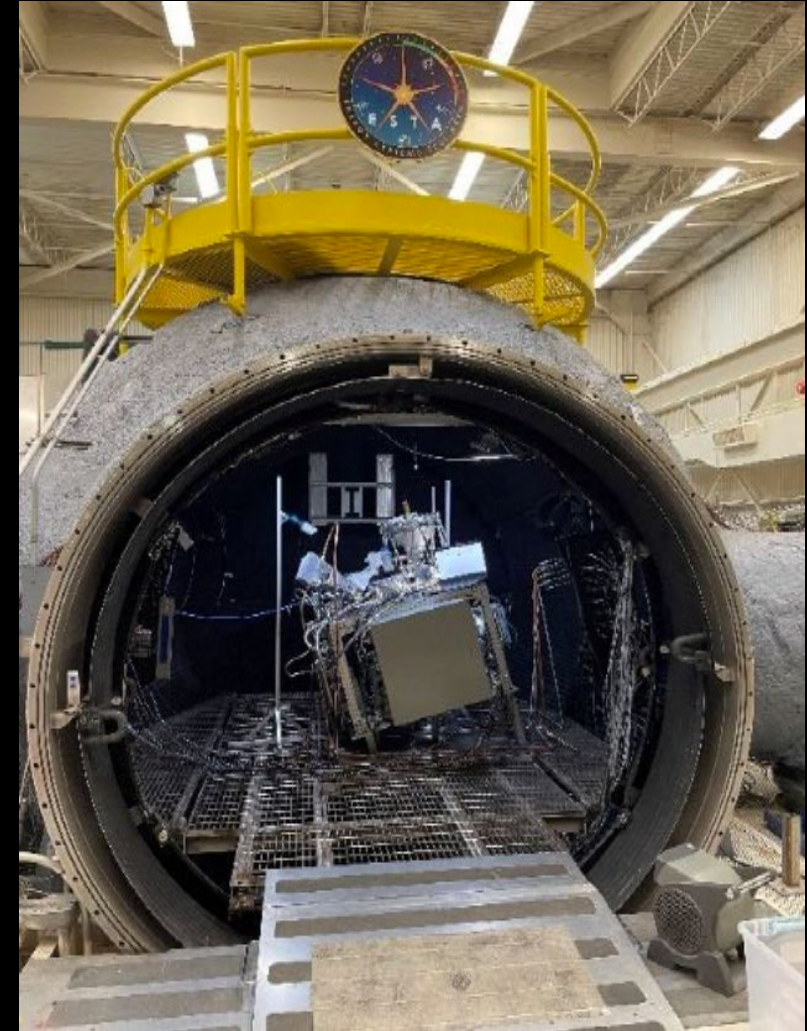
Carbothermal Oxygen Production Reactor (left), Carbothermal Oxygen Production reactor (COPR) Test in 15 ft Dirty TVAC chamber at JSC's Energy Systems Test Area (right)
