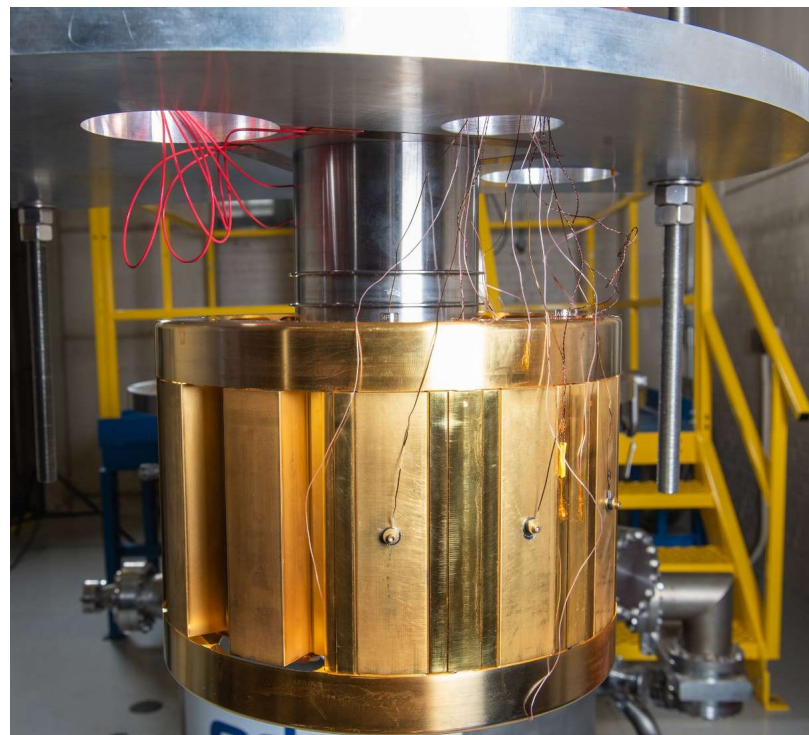
Stationary demonstration of HEMM rotor in TVAC chamber [2]
