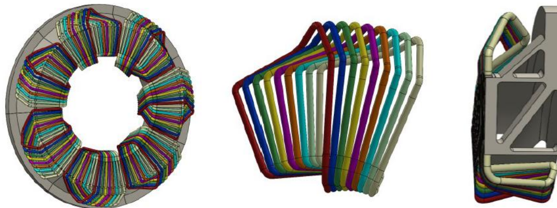
Fig. 3 "Distributed" stator topology. Windings have no skew in the active region of the machine and correspondingly complex end turn geometry.
