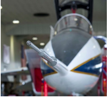
Shock sensing probe mounted on NASA F-15
