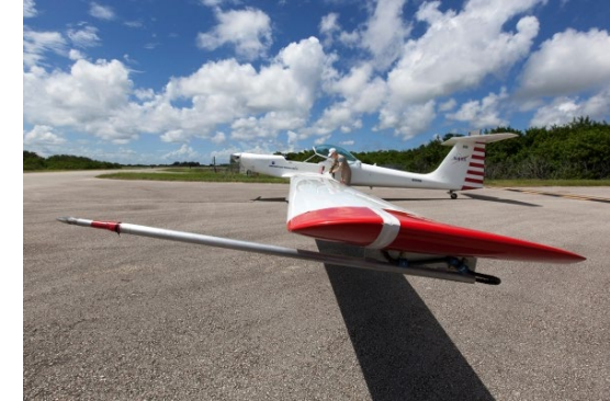
TG-14 motorized glider with wing-tip mounted microphone
