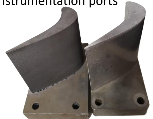
Turbine Blade with integral instrumentation ports
