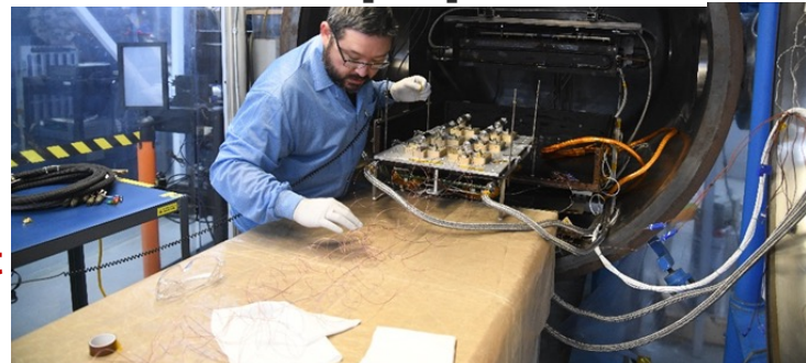
Setting up for TVAC test along with TC read outs
