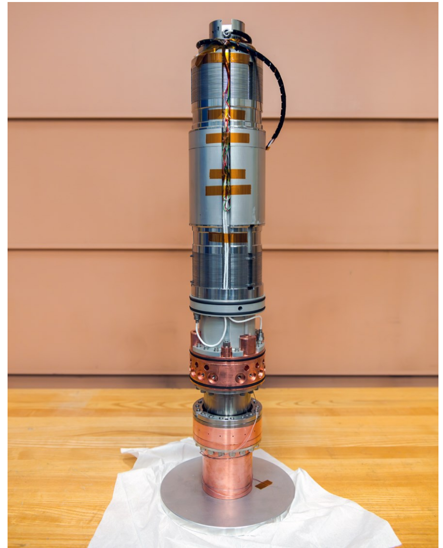
Cryocooler before integration with test stand
