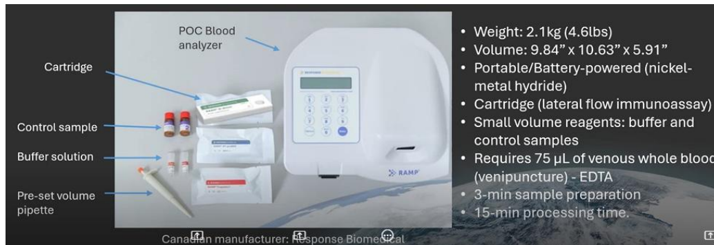
CSA D-dimer hardware prepared for ISS tech demo study
