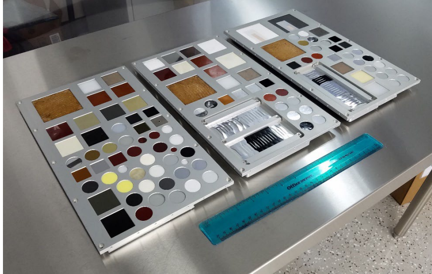
Figure 9. Pre-flight photograph of the MISSE-9 PCE-1 samples loaded into the MSC MS flight decks, from left to right: R2 MSC 3 (ram), W3 MSC 8 (wake), and Z3 MSC 5 (zenith).
