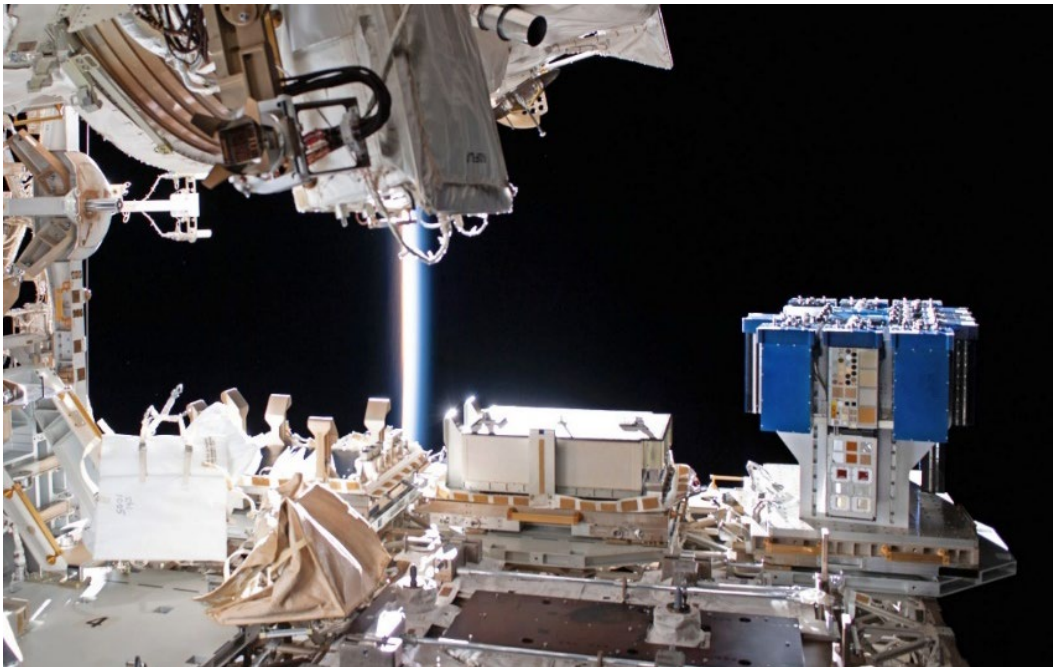
Figure 16. The wake side of the MISSE-FF with the MISSE-10 PCE-2 and MISSE-12 PCE-3 MSCs as photographed on January 25, 2020 during an EVA. The MSCs are closed, except for the central wake MSC which is open (iss061e143021).
