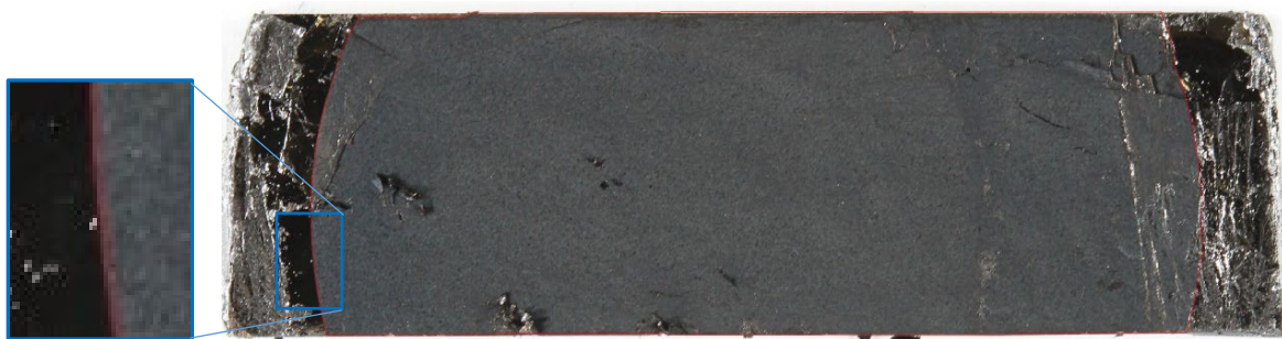
Figure 21. Post-flight photograph of MISSE-9 ram HOPG flight sample (M9R-C22 F) with the AutoCAD ® red line trace used to determine the exposed surface area.
