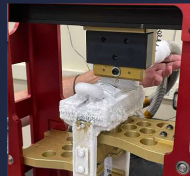
Cryo Cut Test
