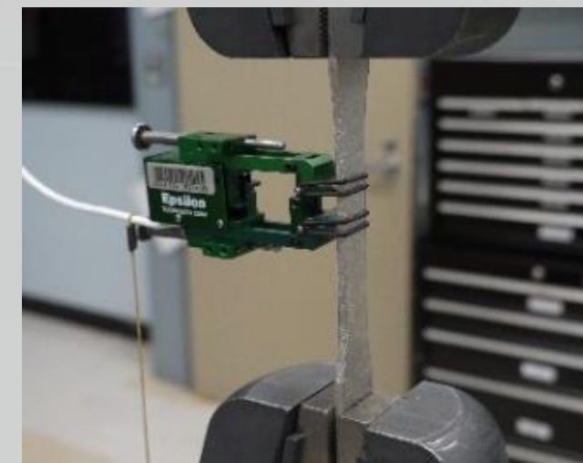
Plated Dog Bone Sample in Tensile Test
