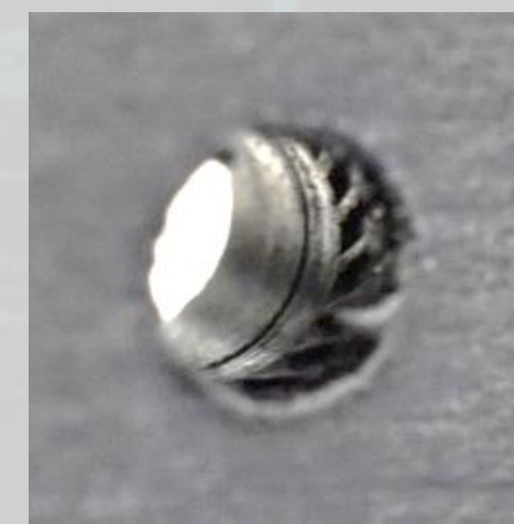
Impression Left in Material from Heat Insert Pull Out
