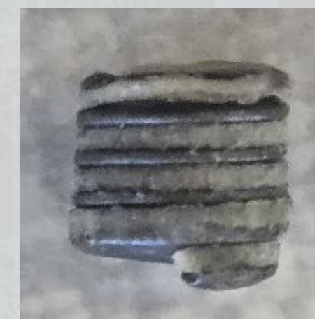
Helical Insert after Pull Out
