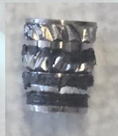
Heat Insert after Pull Out
