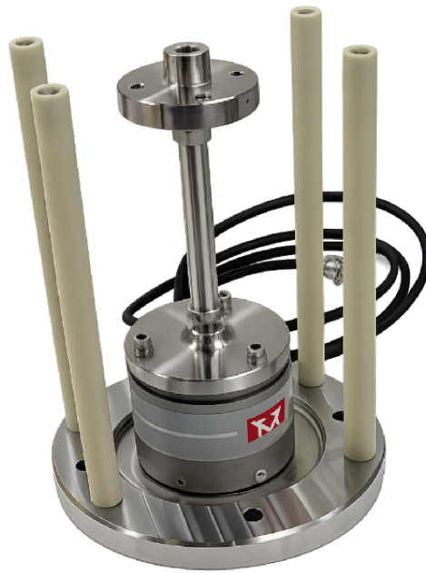
Figure 4. LESTR Unit 01 lower load train and four cold-box support beams.
