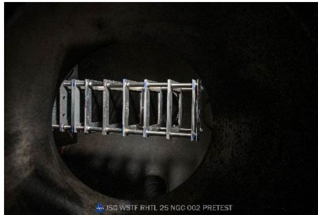
Figure 2-1. A test article showing the 10 membrane layers held in the test fixture and placed in the chamber at WSTF.
