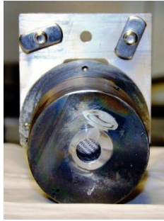
Figure 6. Photo of a laboratory unaligned-grid RPA.
