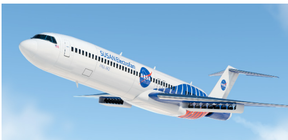
Figure 6. SUSAN showing the 16 wingfans in a mail slot configuration under the wings.
