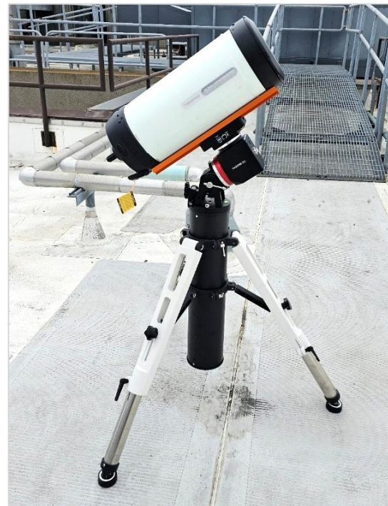
Figure 39: The COTS 20 cm ground station without a detector installed.
