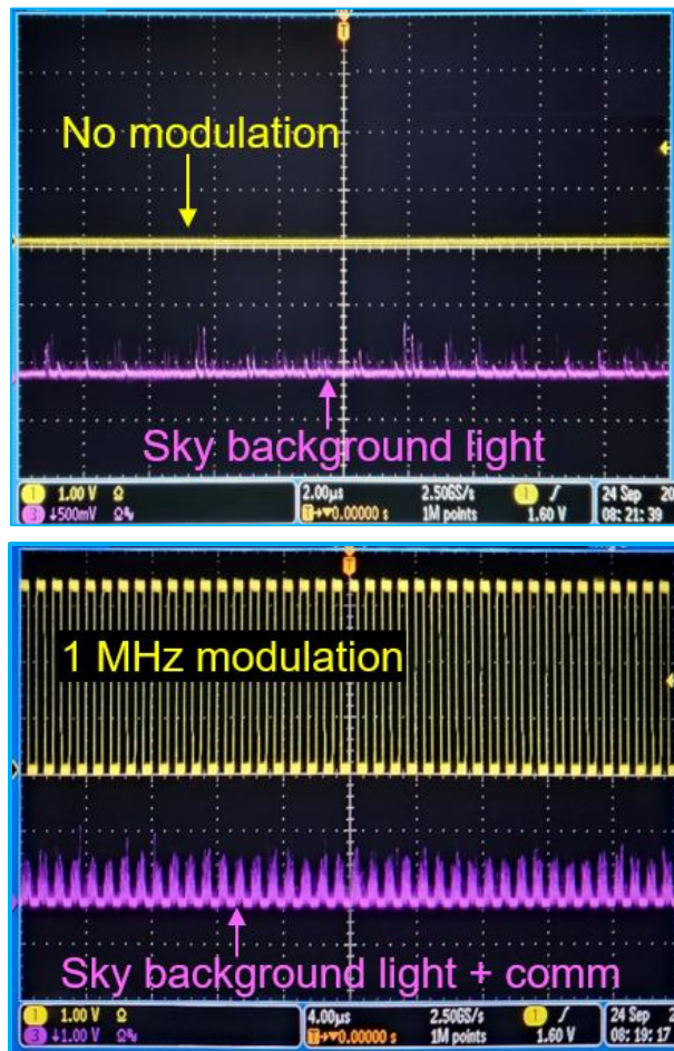
Figure 45: COMLINC optical ground station SNR test in an rural environment; (Top) just background light; (bottom) adds comm signal
