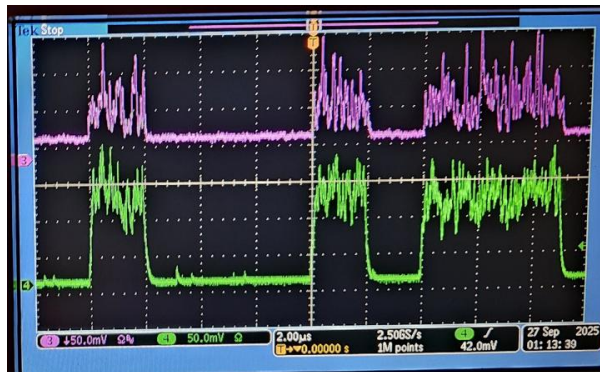
Figure 37: Simultaneous response of the H14951 PMT and C14455 MPPC detectors to a 59 pW avg power, 1 Mbps PRBS signal
