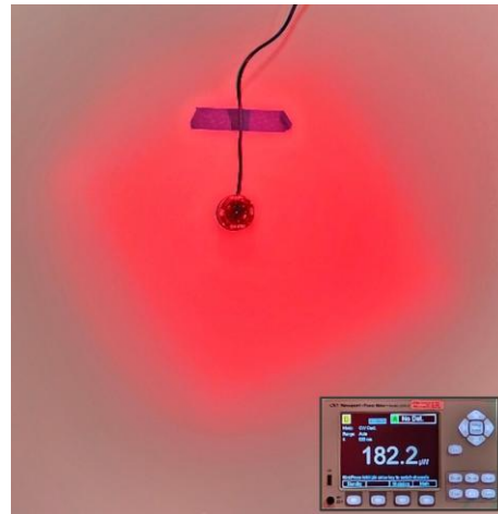
Figure 32: Power in the center of colimated image from the Carclo 10158 lens
