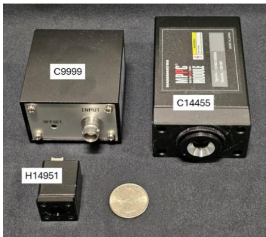
Figure 16: Two Hamamatsu detectors and a transimpedance amplifier
