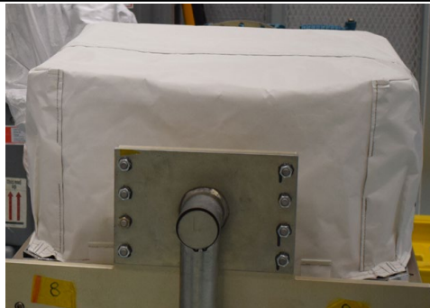
MLI flight blanket fit check.
