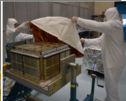
MLI flight blanket fit check.
