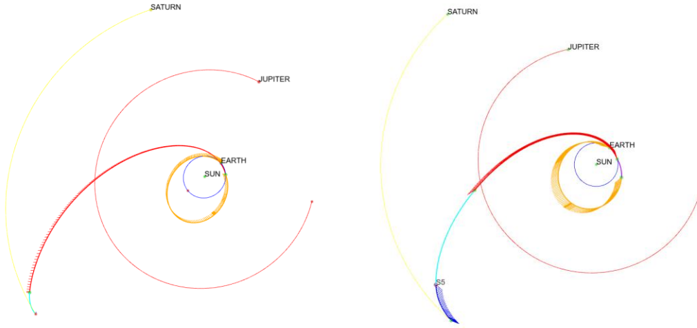
Figure 2. Example of E(2y)ES Minimum Power Trajectories (Left: C_3 = 0 \text{ km}^2/\text{s}^2 , TOF = 1278 days, I_{sp} = 4000 \text{ s} . Right: C_3 = 48 \text{ km}^2/\text{s}^2 , TOF = 3470 days, I_{sp} = 4000 \text{ s} ).
