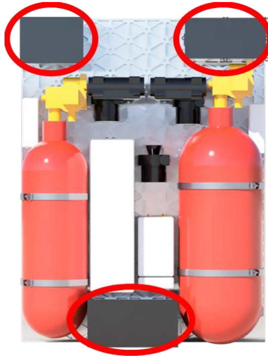
Figure 12.3.1: Avionics Box Locations
