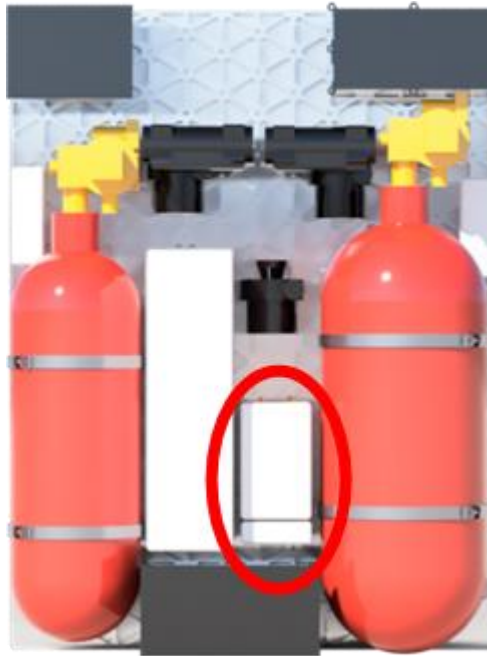
Figure 12.1.1: Solid State Battery Location
