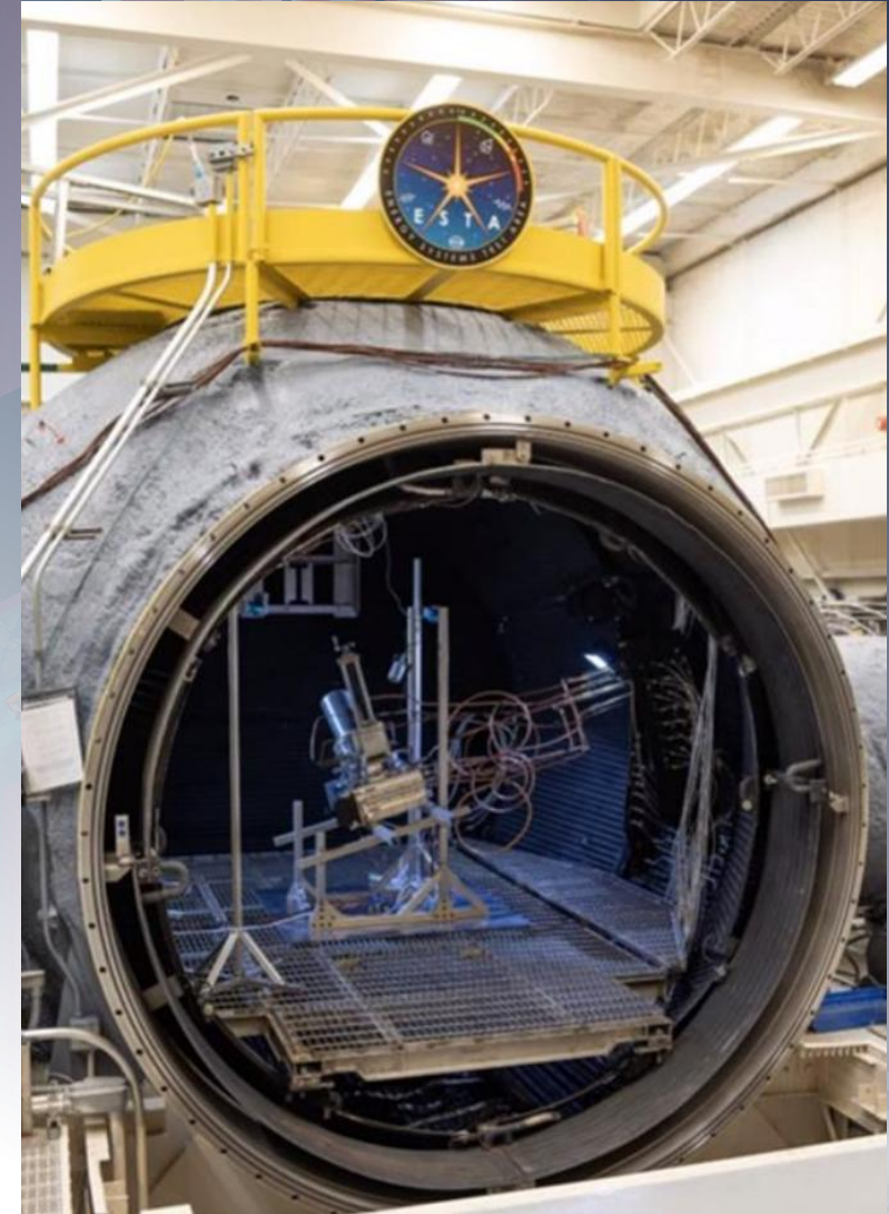
Sierra Space carbothermal reactor in the large thermal vacuum chamber at JSC Energy Systems Test Area.
