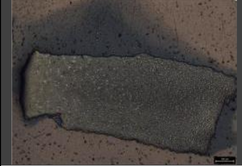
Carbon Mass Cross-Section with Embedded Iron Catalyst Particles
