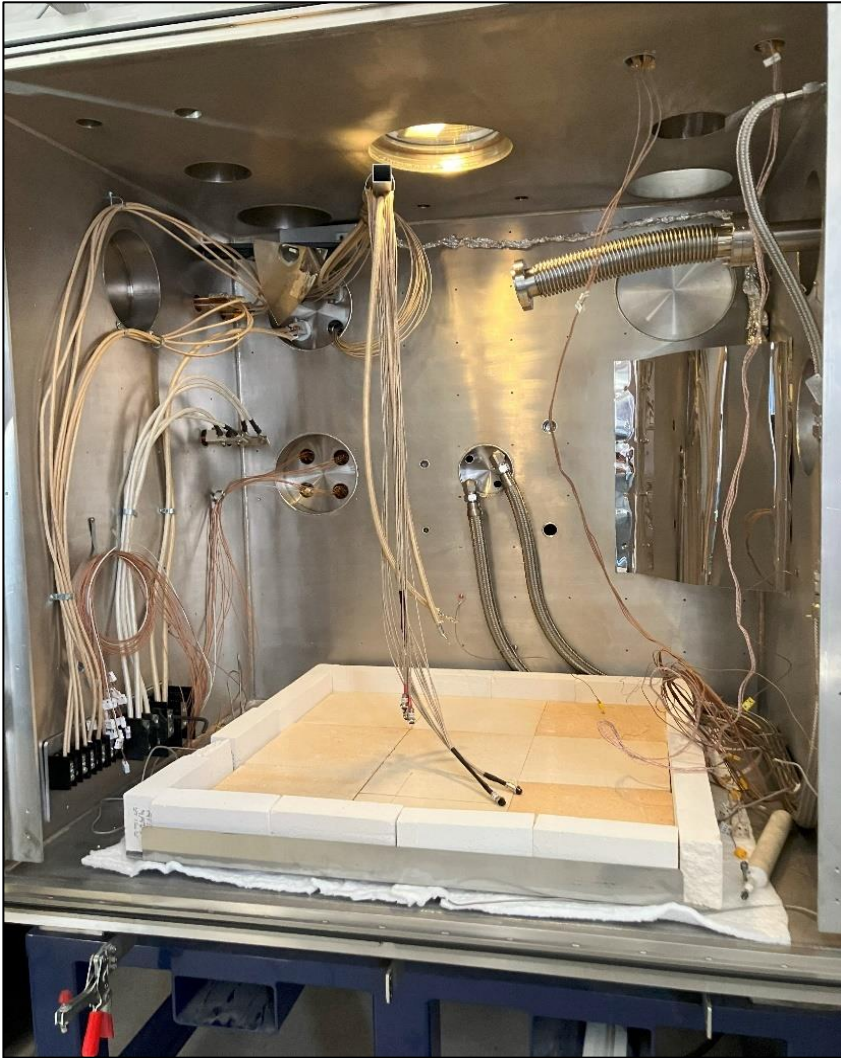
KSC Hardware was quality checked via an XE-6 torr vacuum test.
