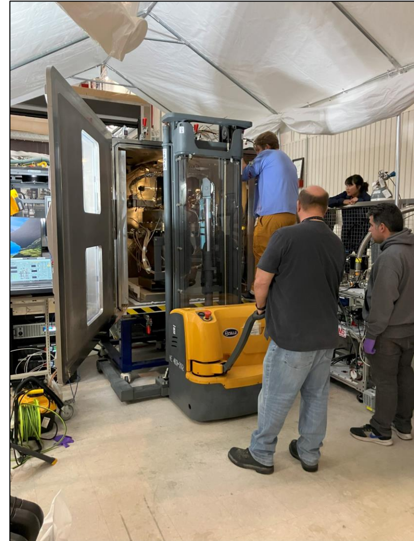
Loading reactor into ASSSIT chamber
