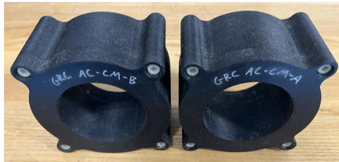
Fig. 3-48. GRC Fabricated AC CM Damping Choke
