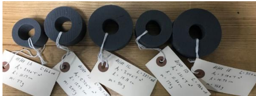
Fig. 3-19. Soft Magnetic Cores from NASA ( B_{max}=0.9T , 80% Stacking)
