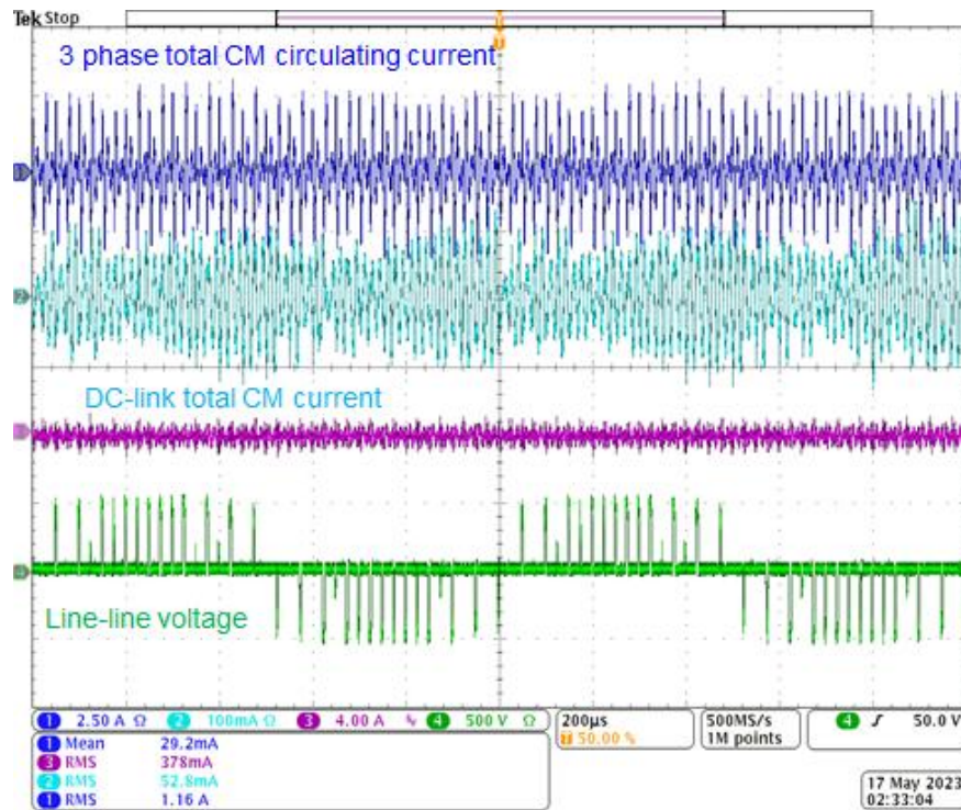
Fig. 3-51. 3-Phase Total CM Circulating Current, DC-Link CM Current, CM Inductor Current and the Line Voltage for the NASA-GRC Cores under 1 kV and M=0.1
