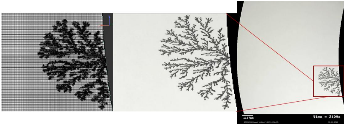
Figure 3-6. Schematic illustration of Adaptive Mesh Refinement (AMR) for Phase-Field simulation of electric tree propagation
