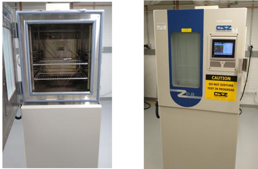
Figure 4-3. Thermal cycling chamber at RTX Technology Research Center (RTRC)
