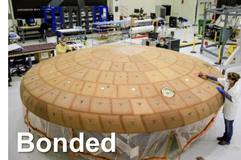
High-temperature Reusable Surface Insulation Tile Attachment System
