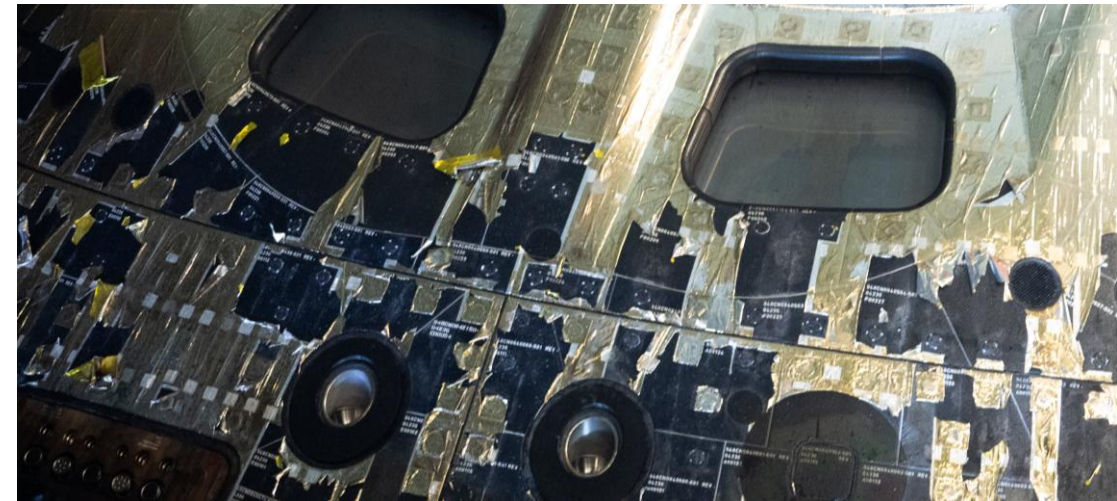
The tape is burnt following flight so this would not be a suitable approach for a TPS that is intended to be reused.
