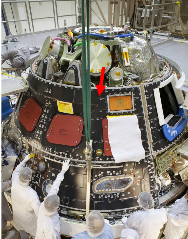
AETB tiles are used as the backshell TPS on Orion
