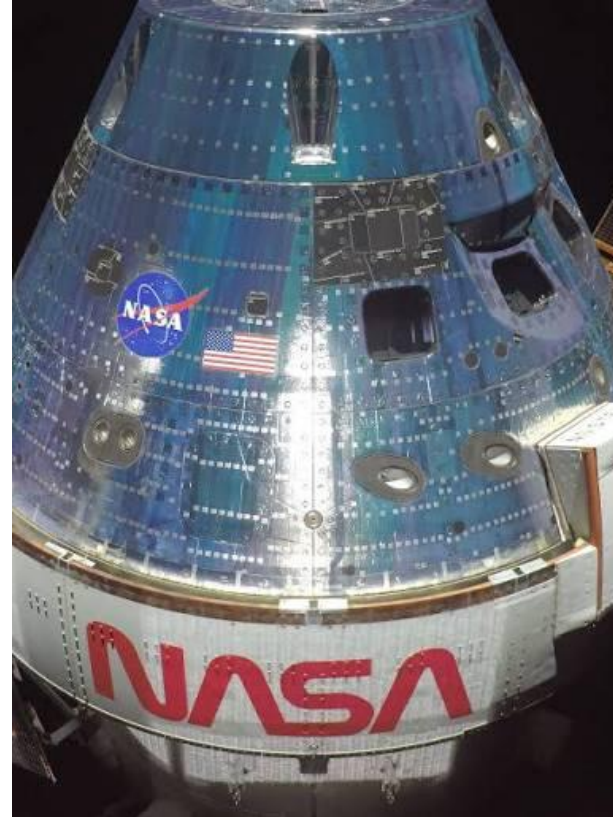
Aluminized thermal tape added for passive thermal control in-space (bondline temp, spacecraft needs) and for electrostatic charge dissipation.
