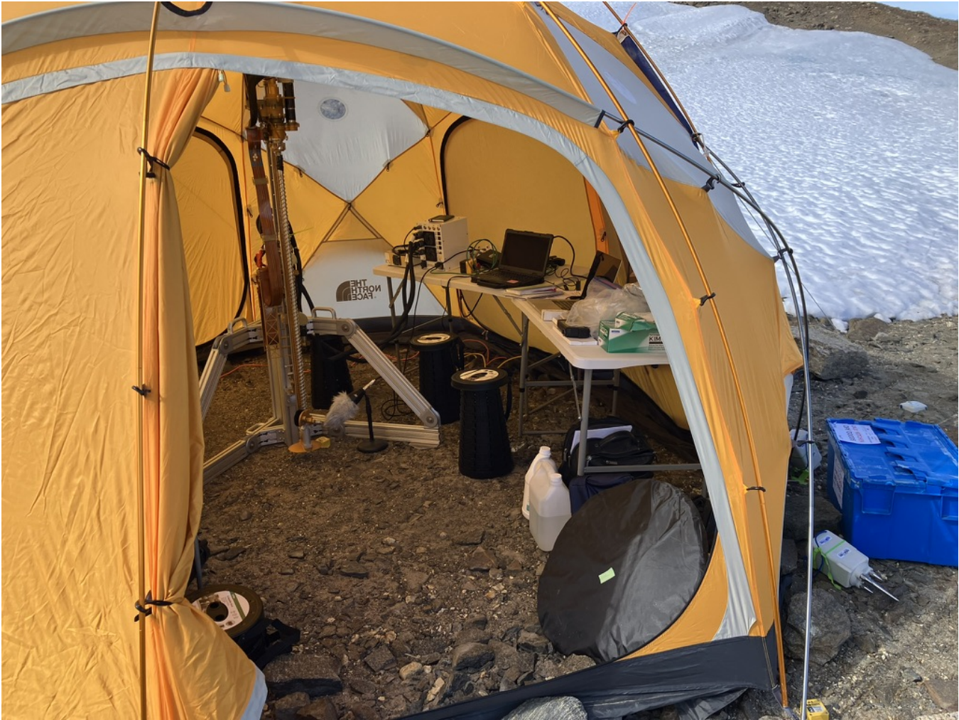
Fig. 7. Drilling into thawed/frozen subsurface boundary in Schirmacher Oasis in Antarctica. Photo credit B. Glass.
