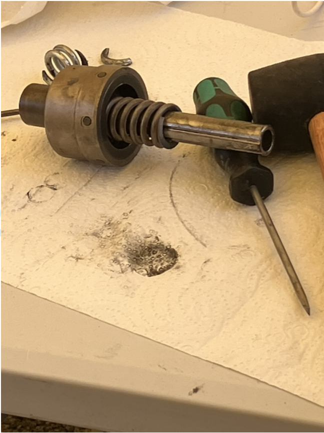
Fig. 13. Replacement for broken percussive spring.
