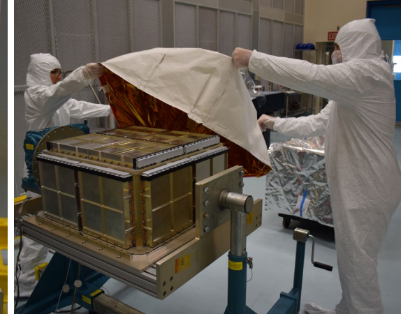
MLI flight blanket fit check.
