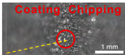
Video 3. The effect of a 250-mph impact on APS Ti/2 vol% hBN coatings, illustrating the chipping and failure of the coating. This video emphasizes the brittleness and reduced durability of the APS coating under extreme impact conditions. A video clip is available online. Supplementary material related to this article can be found online at doi:10.1016/j.triboint.2024.110339 .
