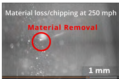
Video 2. A 250-mph impact test on the Ti substrate, where significant material loss is observed. The video showcases how the high-velocity impact results in severe erosion and damage to the uncoated Ti surface. A video clip is available online. Supplementary material related to this article can be found online at doi:10.1016/j.triboint.2024.110339 .
