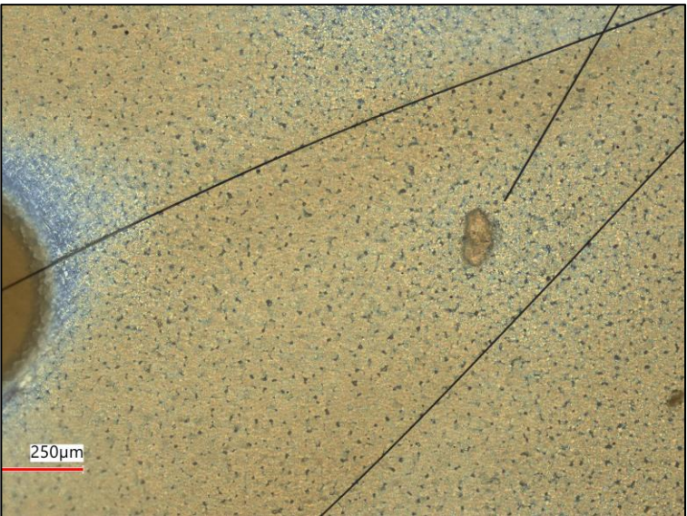
Slow Cooled PEKK: no loss of crystallinity, consistent with both FTIR and DSC data
