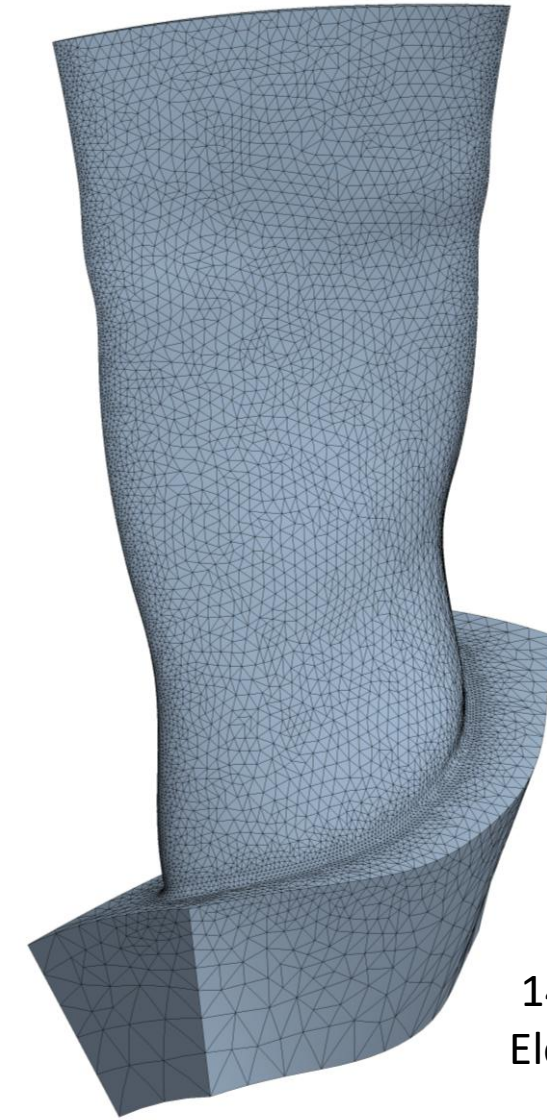
Mesh used for Optimization
