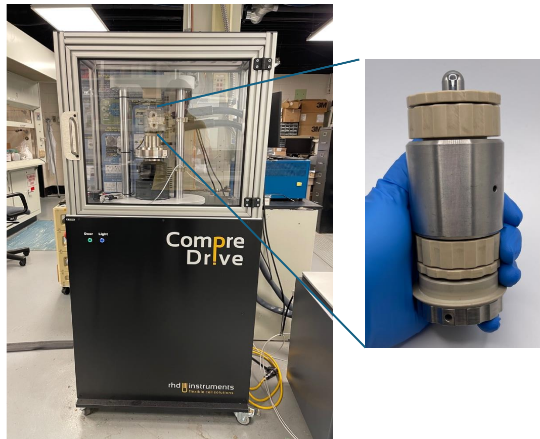
Solid-State Battery Test System with Precise Temperature and Pressure Control
