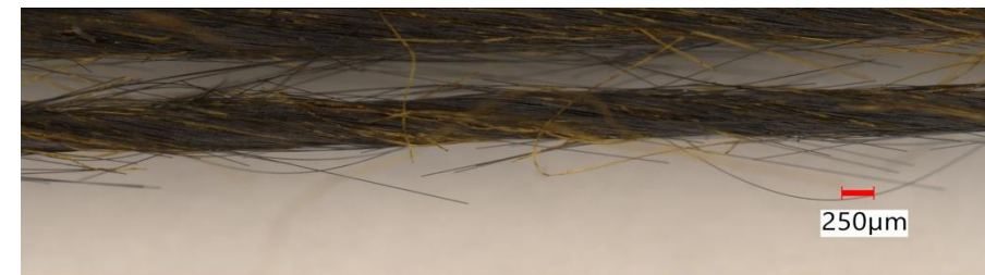
3MDCP single ply image used to obtain ply radius and rotation
