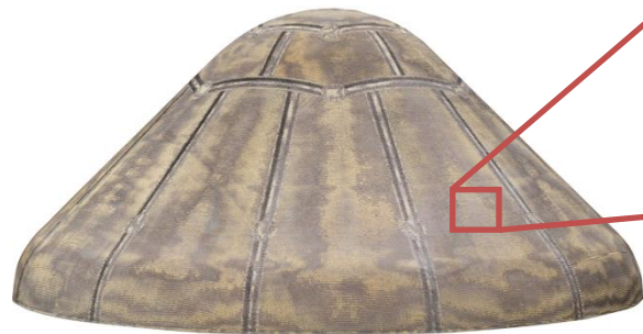
3D Woven Mid-Density Carbon Phenolic (3MDCP)
