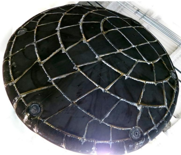
Post-flight heat shields for SpaceX Dragon and Varda W2 capsules.
