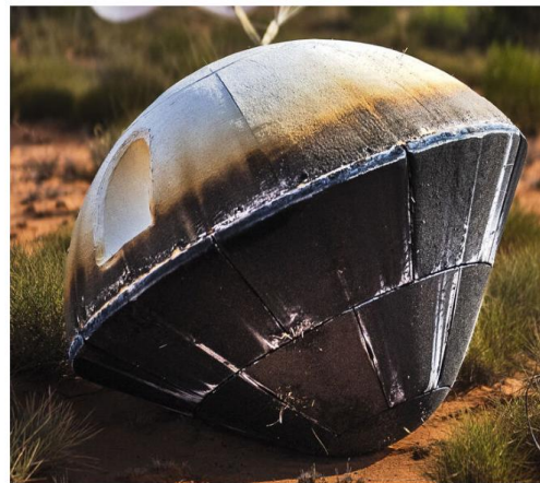
Post-flight heat shields for SpaceX Dragon and Varda W2 capsules.
