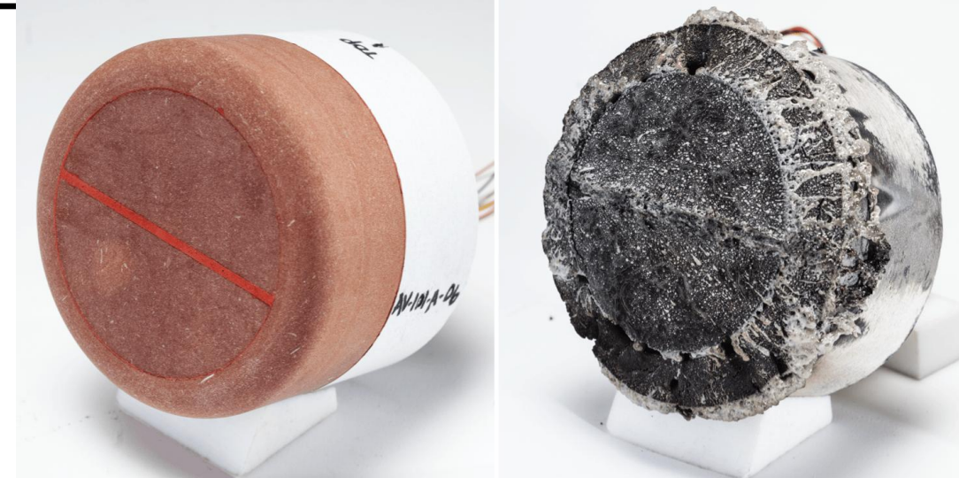
Pre-test and post-test photographs of a flat-face Avcoat test article with RTV-560 gap filler tested at a nominal EM-1 profile for 660 seconds. Source: NASA
