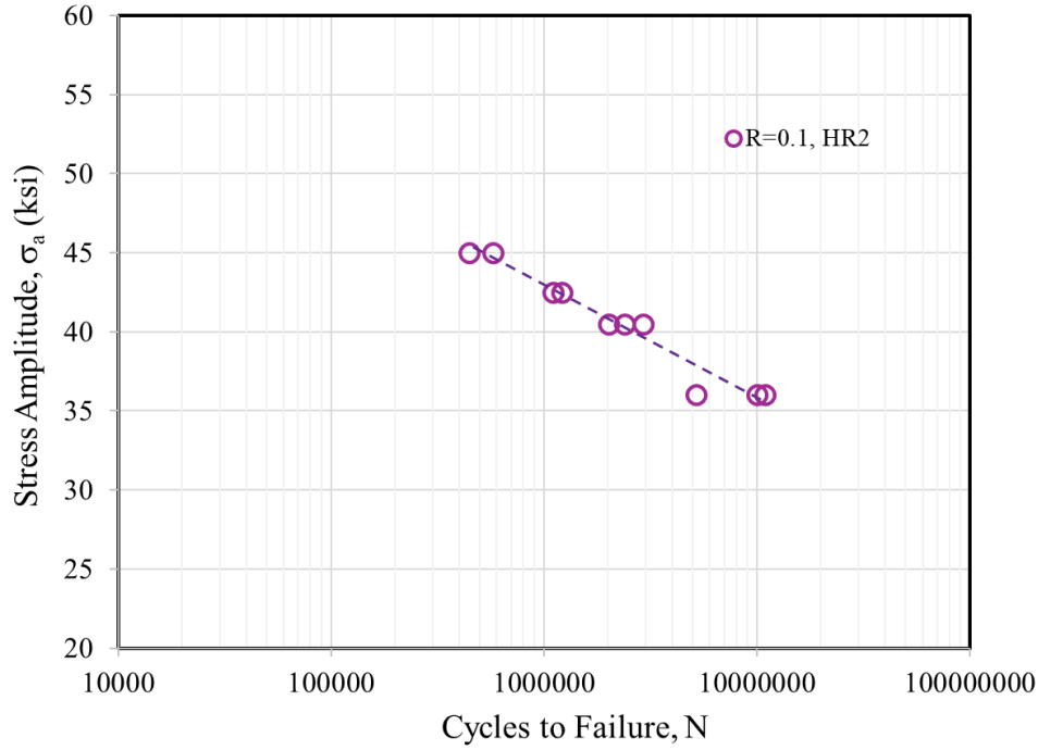
Figure 20. HCF S–N response of machined L-PBF HR-2 at R = 0.1 . Stress amplitude is plotted versus cycles to failure on a logarithmic scale. Runout is defined as 10^7 cycles. The results show a continuous decrease in fatigue life with increasing stress amplitude.
