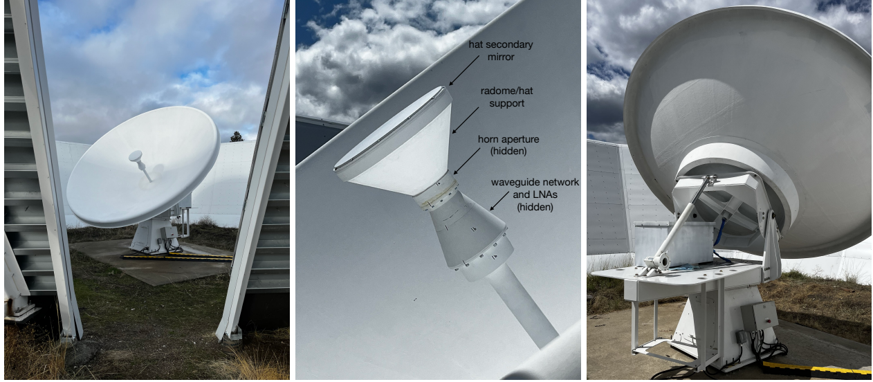
Figure 5. Images of the CGEM optics as they are currently deployed. Left panel: a face-on view of the optics during an azimuth scan. Middle panel: a close-up of the feed column and hat support, with key components labeled. Right panel: a view of the back of the dish to illustrate the ring backing structure on the primary mirror, and the steel cross with set screws that holds the feed column in place. The tree tip visible over the ground shield in the photo at left is not visible from the location of the telescope.
