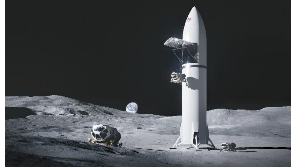
Figure 14. Artist's concept of the Starship HLS autonomous cargo lander, capable of delivering 15 mT of payload to the lunar South Pole to support NASA's goals for sustainable exploration. (Credit: SpaceX)
