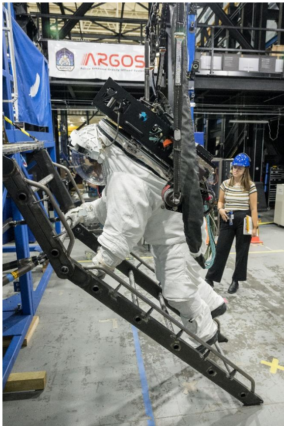
Figure 4. Blue Origin conducted testing using the Active Response Gravity Offload System (ARGOS) test fixture at NASA Johnson to evaluate ladder functionality during suited crew operations.
