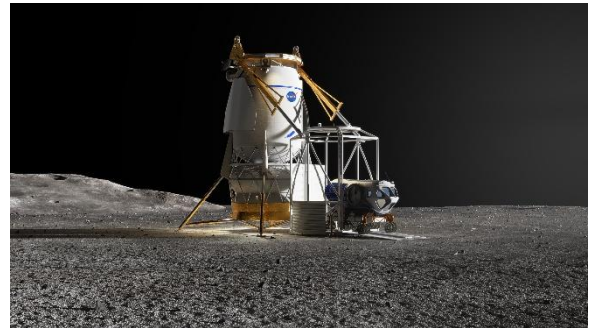
Figure 15. Artist's concept of the Blue Origin Blue Moon MK2 HLS lander for large cargo, such as an initial surface habitat. (Credit: Blue Origin)
