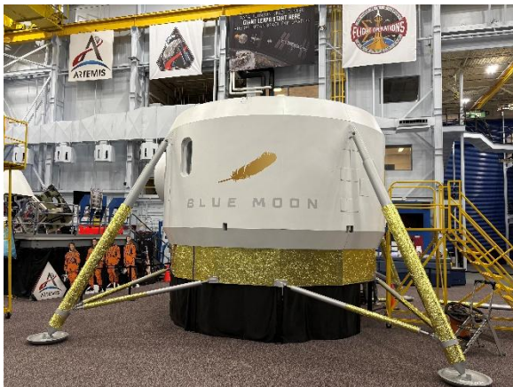
Figure 13. Blue Origin installed a prototype crew cabin of its Blue Moon MK2 HLS at NASA Johnson, which will be gradually outfitted for flight training and other evaluation tasks.
