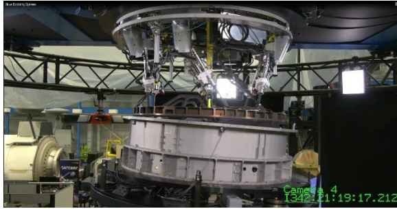
Figure 12. In preparation for Artemis III, Blue Origin successfully completed soft capture testing of its Blue Docking System at the Six-Degree-Of-Freedom (6-DOF) Dynamic Test facility at NASA Johnson. (Credit: Blue Origin)
