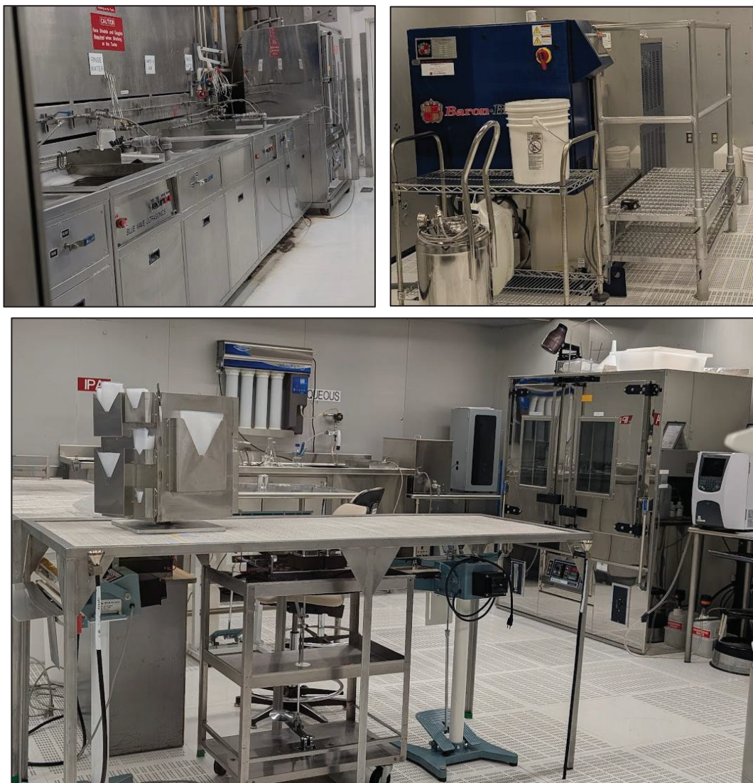
Figure 12. WSTF Cleaning Services Shop: Aqueous Detergent Ultrasonic Baths (Top Left), HFE-7100 Vapor Degreasing System (Top Right), and Precision Cleaning Processing Area (Bottom)
