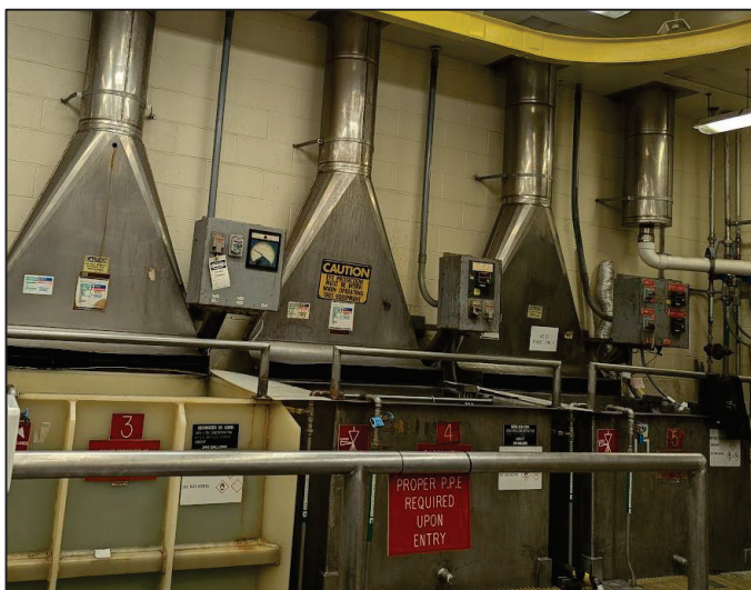
Figure 7. JSC Cleaning Shop Aqueous Ultrasonic Baths (Left) and Pre-Clean/Passivation Tanks (Right)
