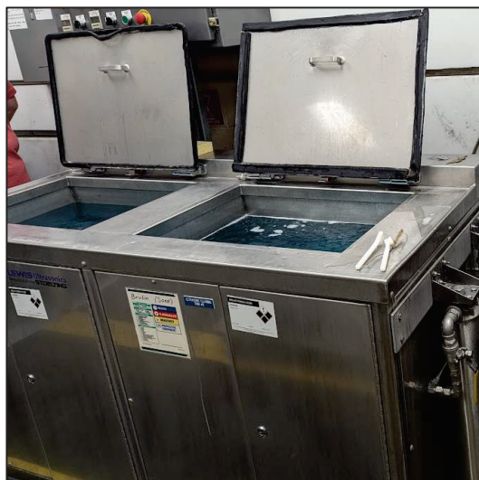
Figure 7. JSC Cleaning Shop Aqueous Ultrasonic Baths (Left) and Pre-Clean/Passivation Tanks (Right)
