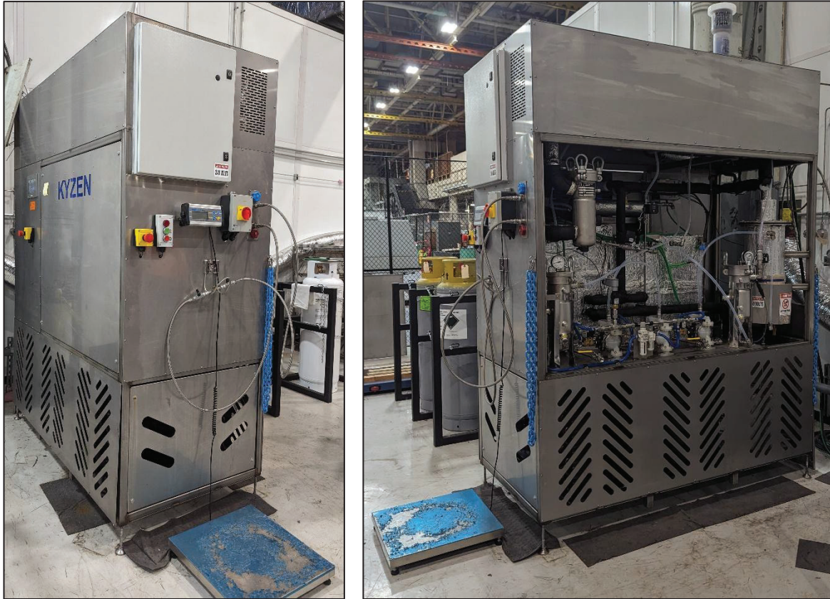
Figure 5. Kyzen Solstice Distillation System at MAF
