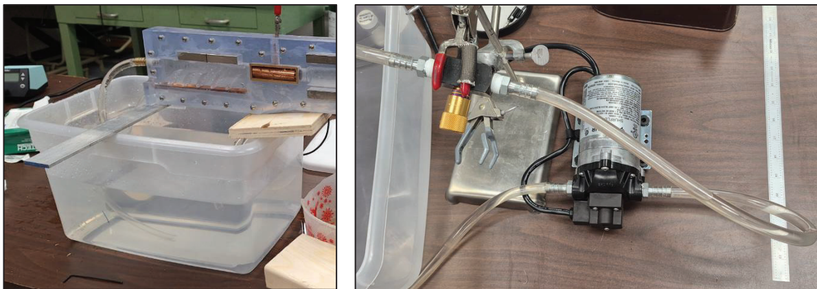
Figure 46: Reservoir bin filled with water with pump inlet line (Left) and pump/control valve (Right).
