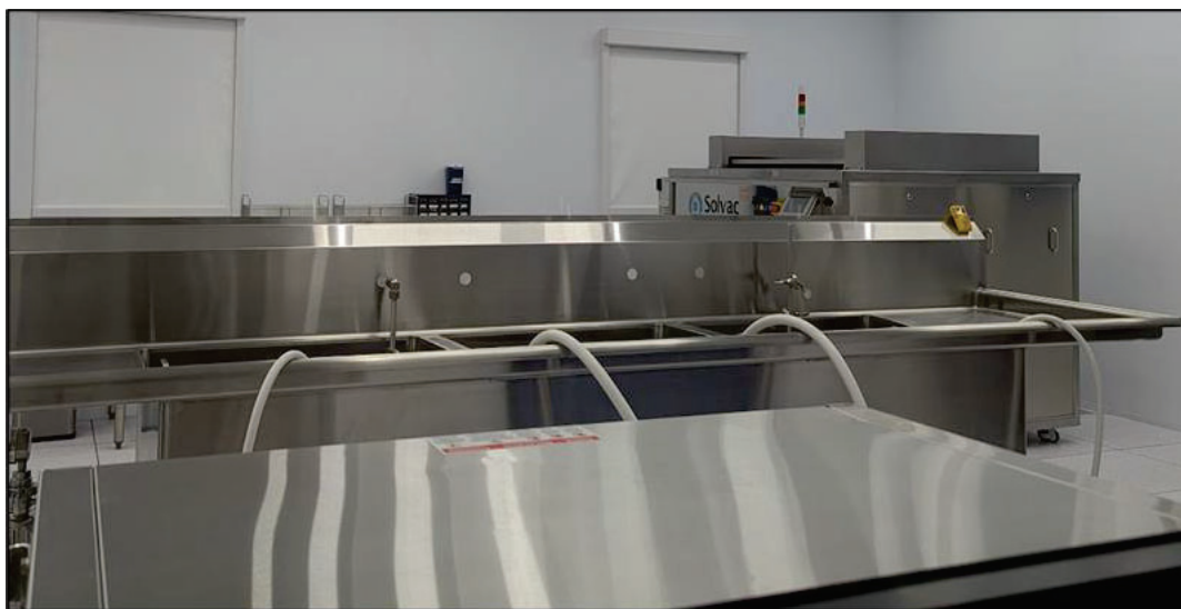
Figure 8. JSC Cleaning Shop Vapor Degreasing System and ISO Class 6 Cleanroom Area
