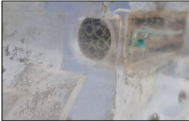
Figure 43. Charged copper tubes bundle within ICAF (side view).
