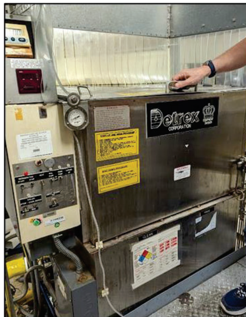
Figure 11. MSFC Valve Shop Vapor Degreaser
